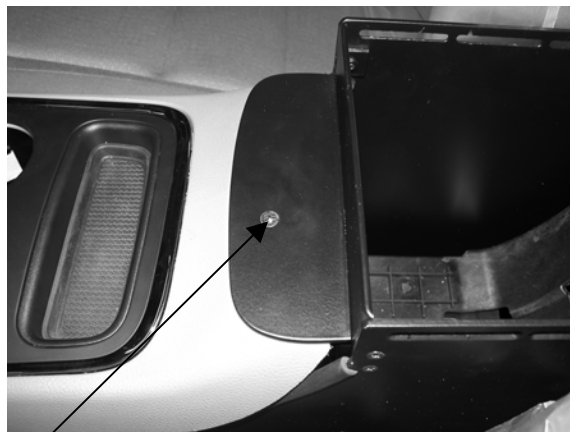
Secure front of Lund console w/ supplied hardware
