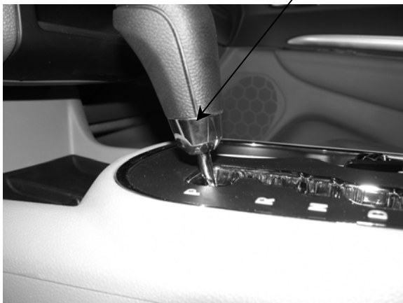
Carefully remove chrome bezel
