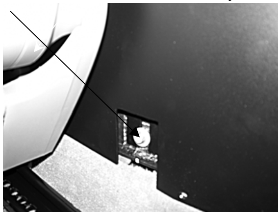
Secure sides of Lund console w/ 2 factory bolts (1 on ea. side)
